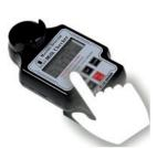
Press the «TEST» button again in order to display the difference in electrical conductivity (DIF).
